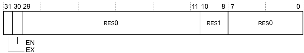
Figure 2-6 FPEXC32_EL2 bit assignments
