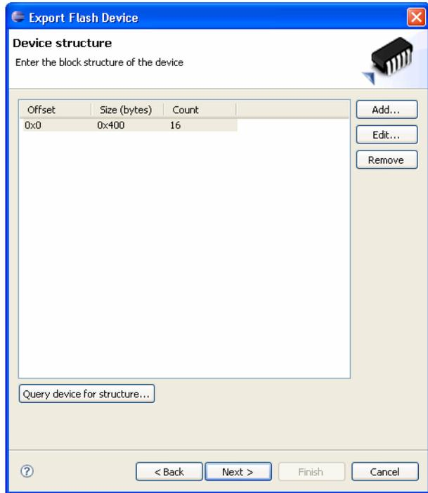
**Figure 14 Describing the block structure of the device**
