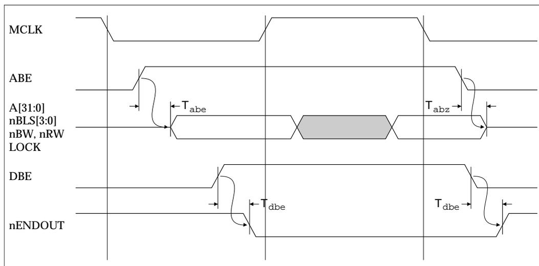
Figure 14-3: ARM710a macrocell bus enable timing
