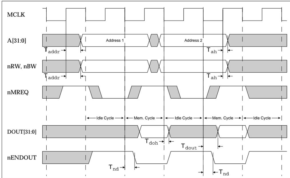
**Figure 11-17: Two single word non-sequential buffered writes**
