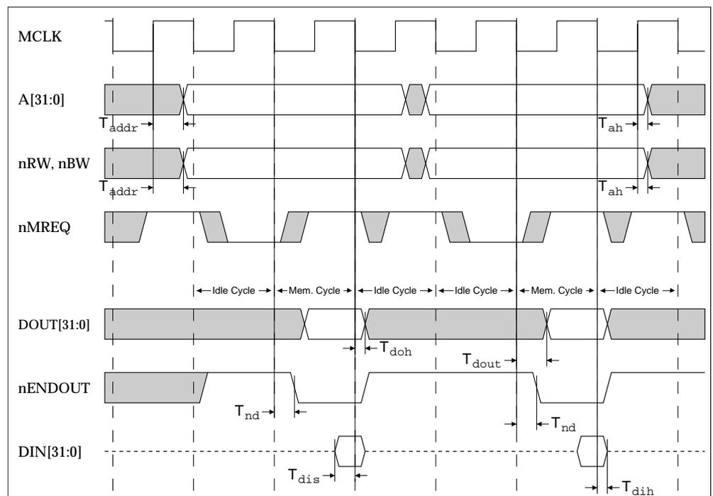
Figure 11-16: Two single word non-sequential unbuffered accesses
