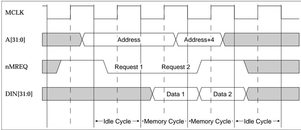
**Figure 11-2: Simplified sequential access**
