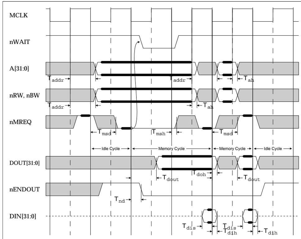
Figure 11-12: Sampling points at maximum frequency
