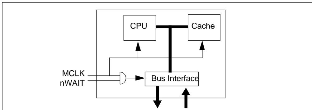
*Figure 10-1: Conceptual device clocking using the fastbus extension*
