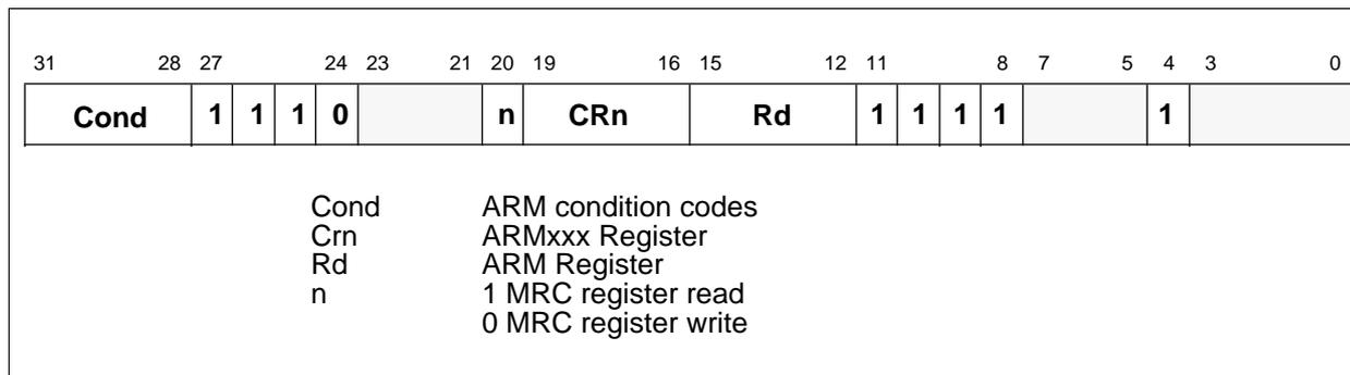
**Figure 5-1: Format of internal coprocessor instructions MRC and MCR**
