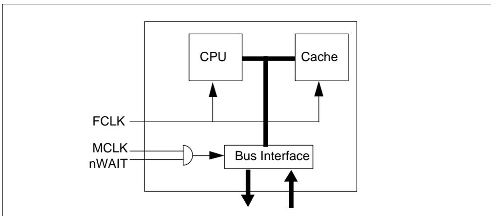
**Figure 10-2: Conceptual device clocking in standard mode**
