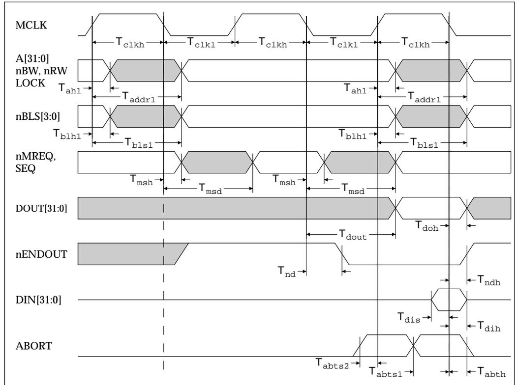
Figure 14-1: ARM710a macrocell bus timing, ALE HIGH
