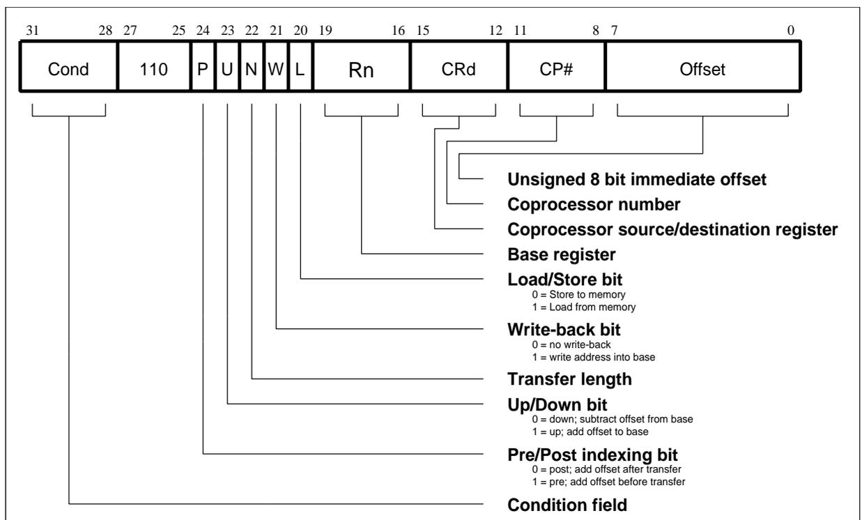
Figure 4-23: Coprocessor data transfer instructions
