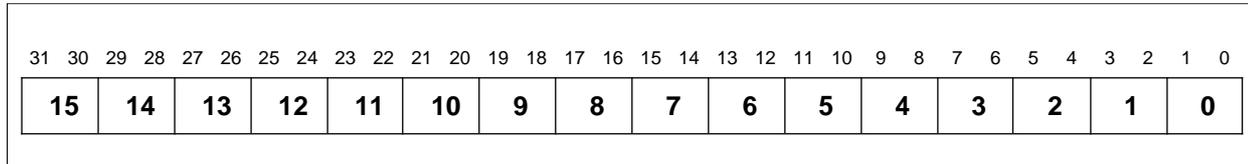
**Figure 9-9: Domain access control register format**
