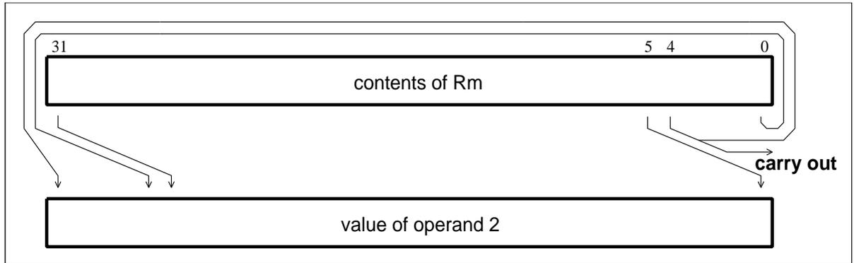
**Figure 4-9: Rotate right**
