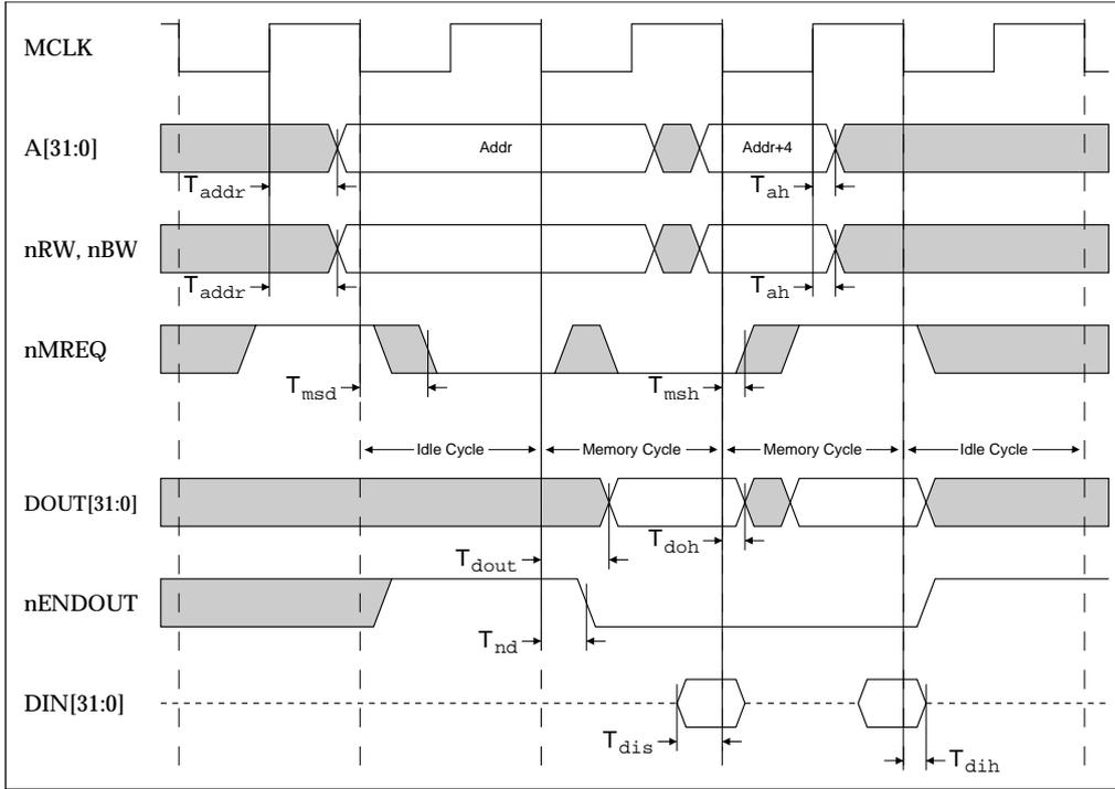
**Figure 11-4: Two word sequential read or write**
