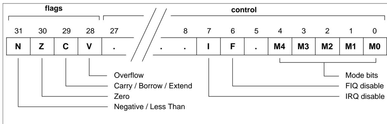
**Figure 3-4: Format of the program status registers (PSRs)**
