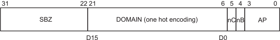
Figure B-13 Rd format, RAM1 write
