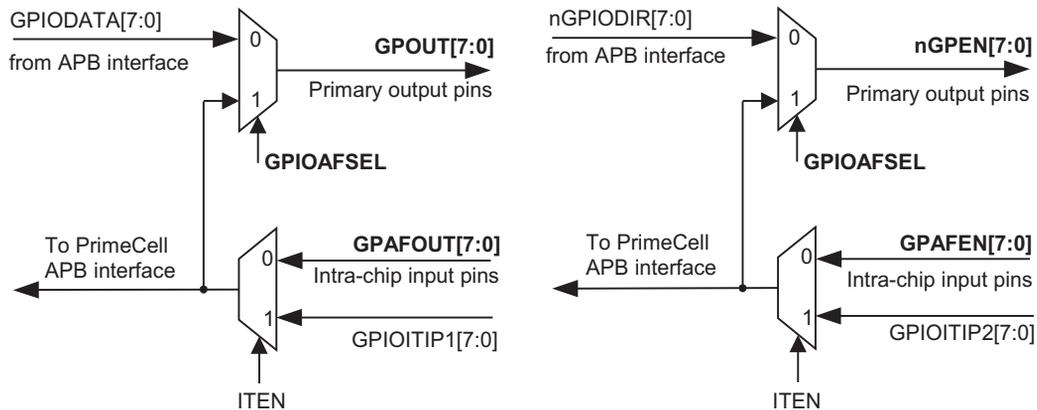
**Figure 4-3 Output integration test harness, primary outputs**
