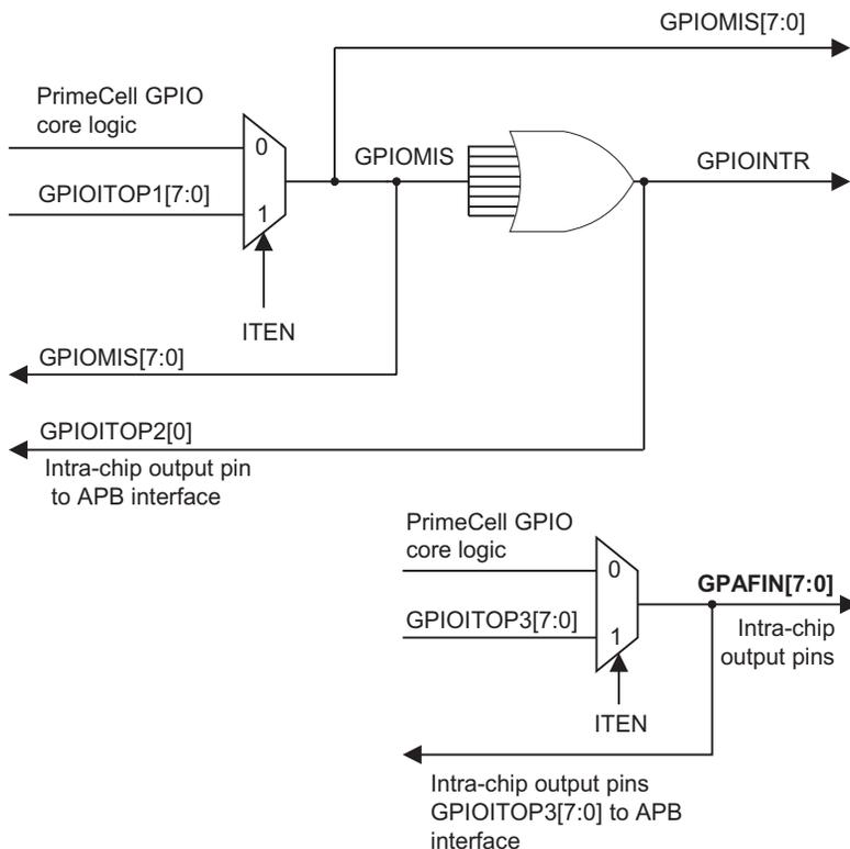
Figure 4-2 Output integration test harness, intra-chip outputs
