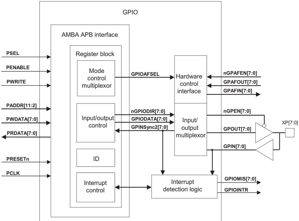
**Figure 2-1 PrimeCell GPIO block diagram**
