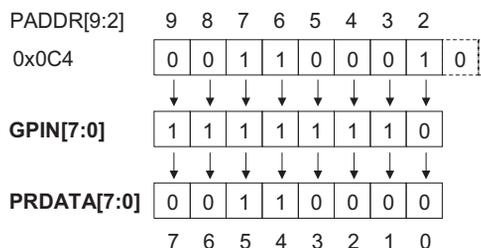
**Figure 2-3 Example 2 Read from address 0x0C4**
