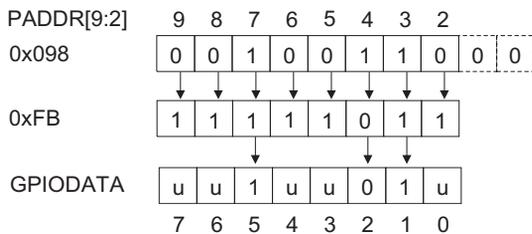
**Figure 2-2 Example 2 Write to address 0x098**
