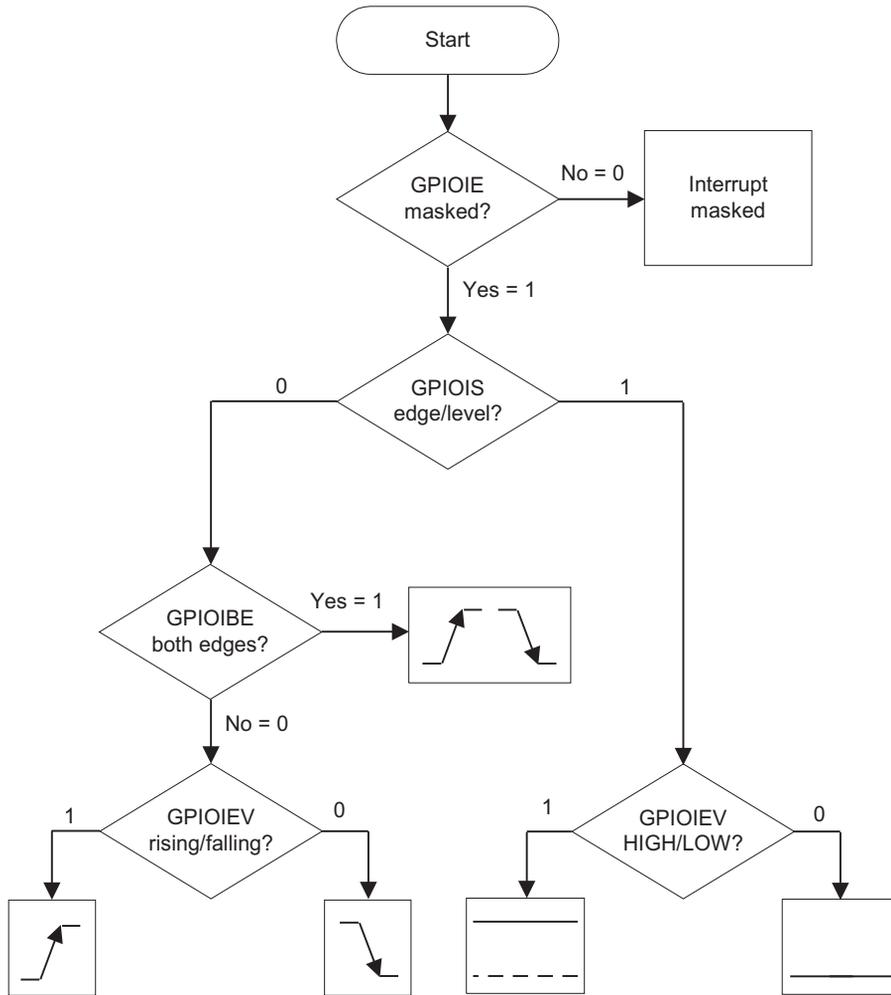
**Figure 2-5 PrimeCell GPIO interrupt registers**
