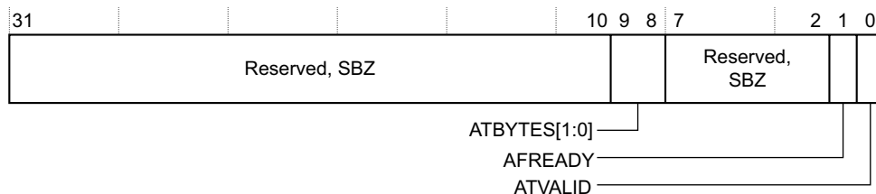
Figure 3-20 ITATBCTR0 Register bit assignments
