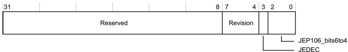
Figure 3-45 PERIPHD2 Register bit assignments
