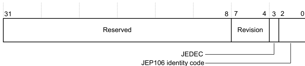
Figure 3-21 SMMU_PIDR2 register bit assignments
