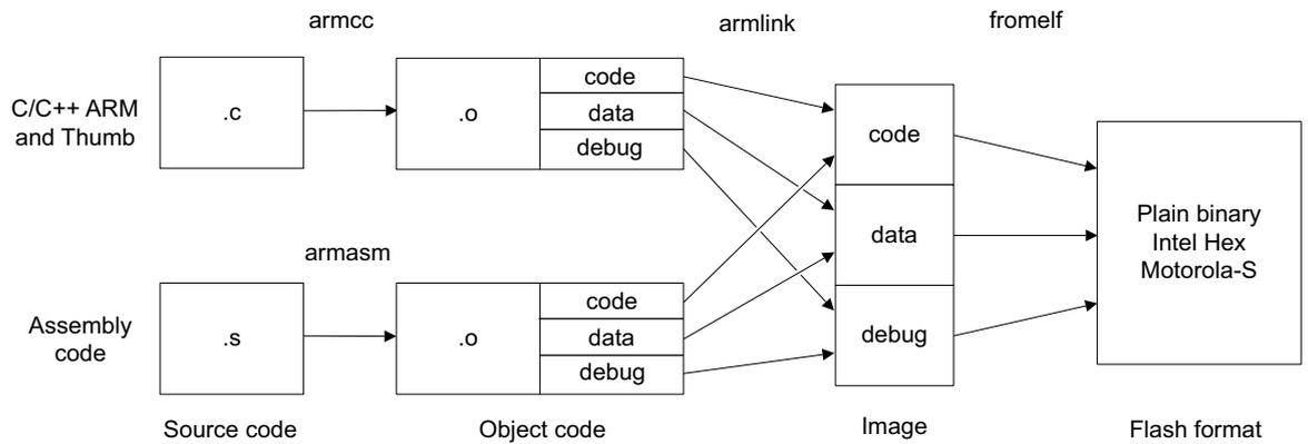
**Figure 3-1 A typical tool usage flow diagram**
